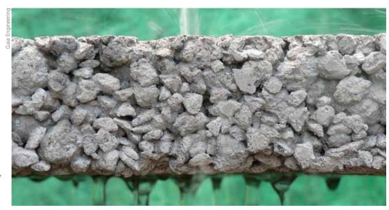
Pervious pavement allows water from precipitation to pass directly through, thereby reducing the runoff from a site and allowing groundwater recharge.
